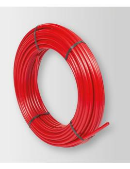
It is available in 12mm, 17mm and 20mm diameters and is compatible with most MYSON FLOORTEC heating systems, including MICROBOARD, our low-profile heating system. It is environmentally friendly and is produced with no chemical additives in either the production or disposal processes. It is quality guaranteed for 10 years and conforms to DIN4726 and BS7291-1:2001.
