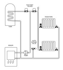
Choose a suitable position for the valve in the circuit to be controlled, which allows sufficient access for wiring and maintenance.
