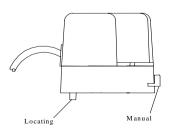
Position the actuator on the valve body by locating the spindle in the cam slot.
